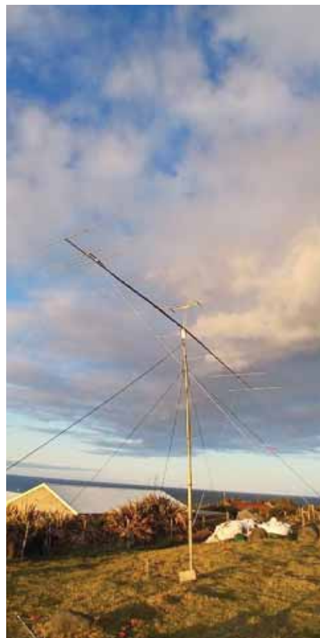
Lance Collister's, W7GJ, 6-meter Yagi at ZD9GJ tied down for moonrise. [Photo courtesy of W7GJ]
