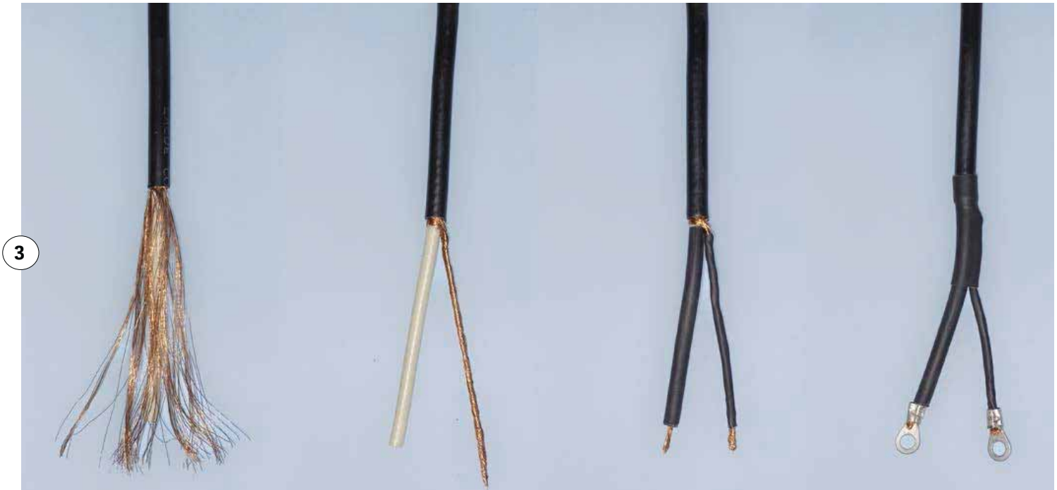
Steps in preparing the feed-point end of the coaxial cable.
