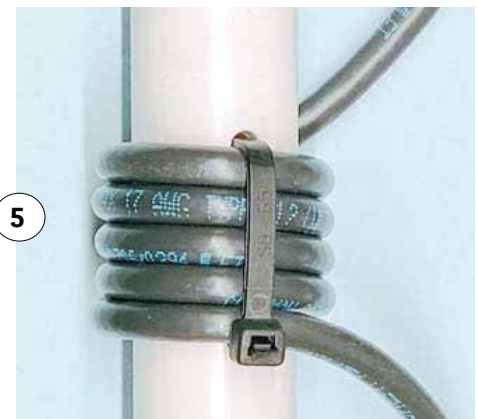
Coax looped down and formed into a balun.
