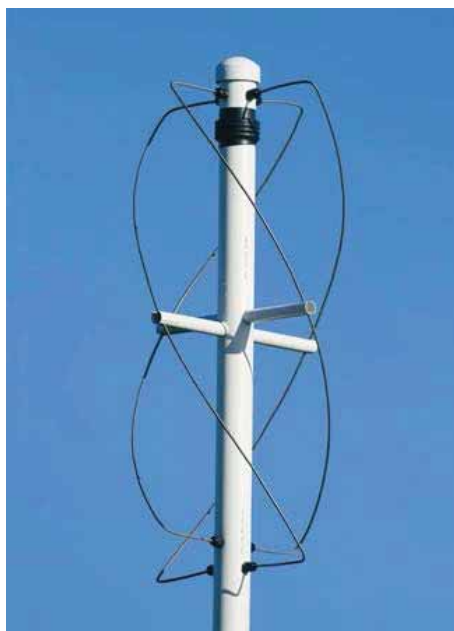
A quadrifilar antenna for 2 meters. [Phil Harris, photo]
