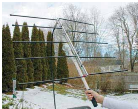
This handheld LPDA antenna is used for satellite operating. [Steve Ford, WB8IMY, photo]
