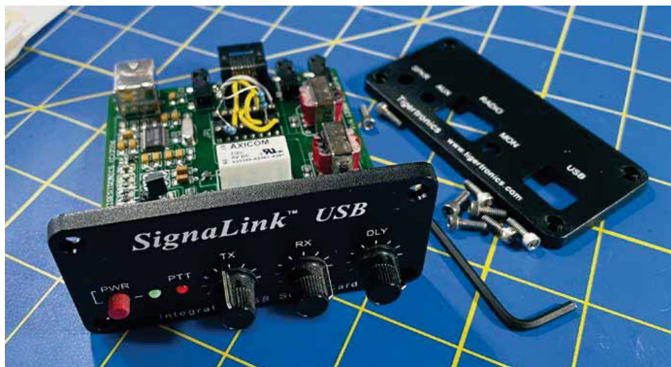
The Tigertronics Signalink with the cover removed to show the inner workings.
