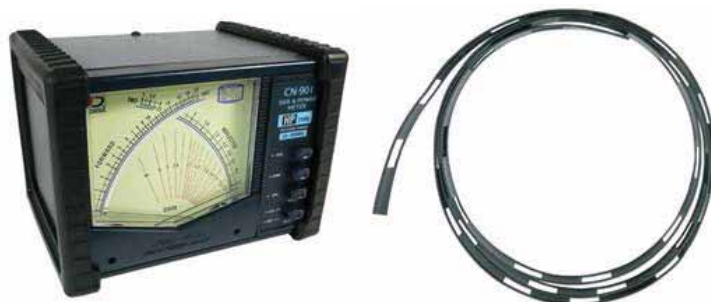
Above: A dedicated external SWR/power meter. Right: Windowed ladder line has extremely low RF loss, even when the SWR is quite high. [DX Engineering photos]
