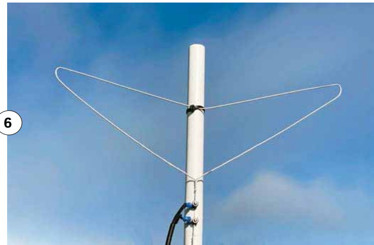
One of the two hangers bent equally inward to raise the antenna's frequency (bend it outward to lower the frequency).
