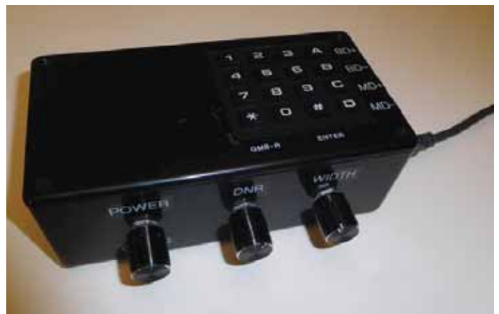
Figure 1 – This Yaesu FT-891 control box has a 4×4 keypad for direct frequency input, a dedicated band button and a dedicated mode button.
