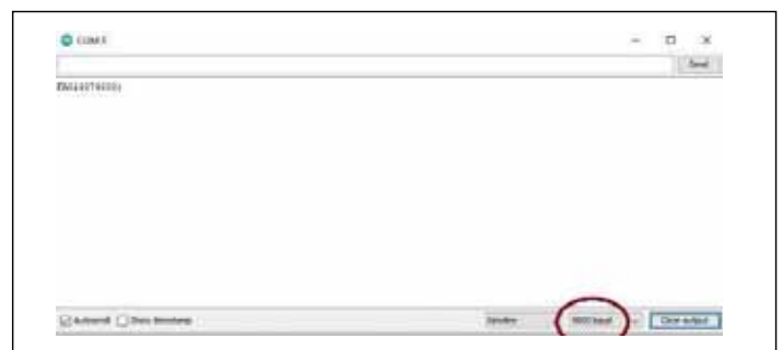
Figure 4 – Here is what you should expect on your screen when entering a 5-digit frequency like 14074 and pressing the ‘#’ Enter key.
