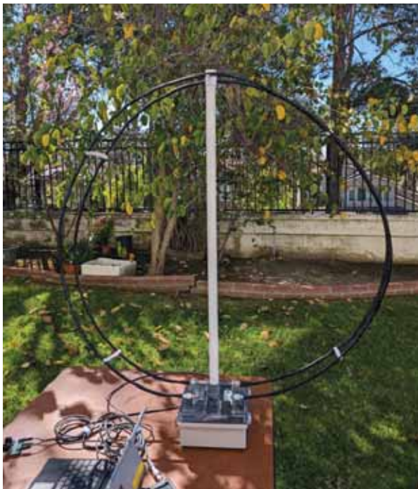
Figure 1 – Desktop MLA setup in the back yard of W6SI.
