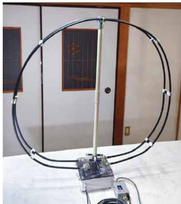
Figure 3 –Two loops, 1 m diameter configuration of Desktop MLA.
