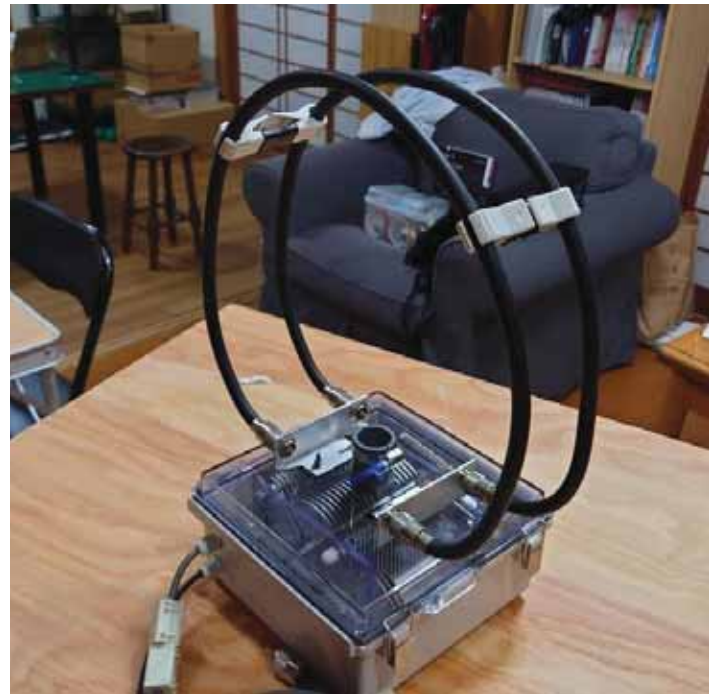
Figure 6 – Two loop, 30 cm diameter configuration for 6 m band.
