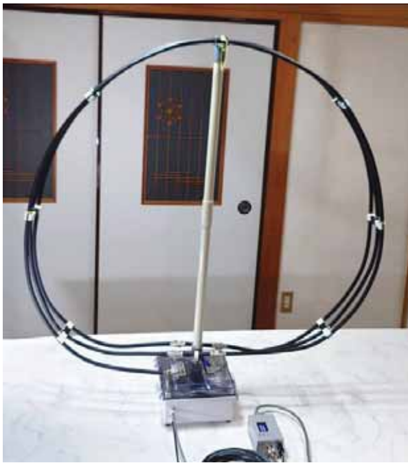
Figure 7 – Single three-turn loop configuration for 80 m band.
