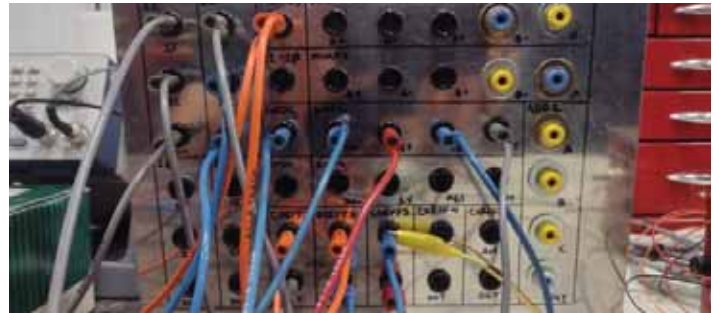
Figure 4 – Analog computer patch panel.
