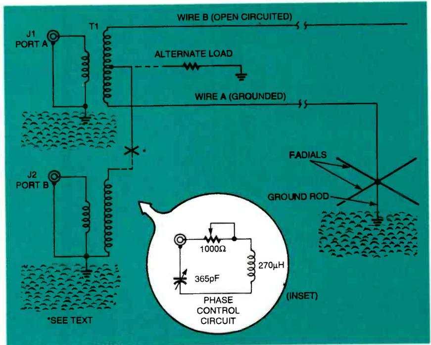
Fig. 10. Steerable-notch Beverage antenna.
